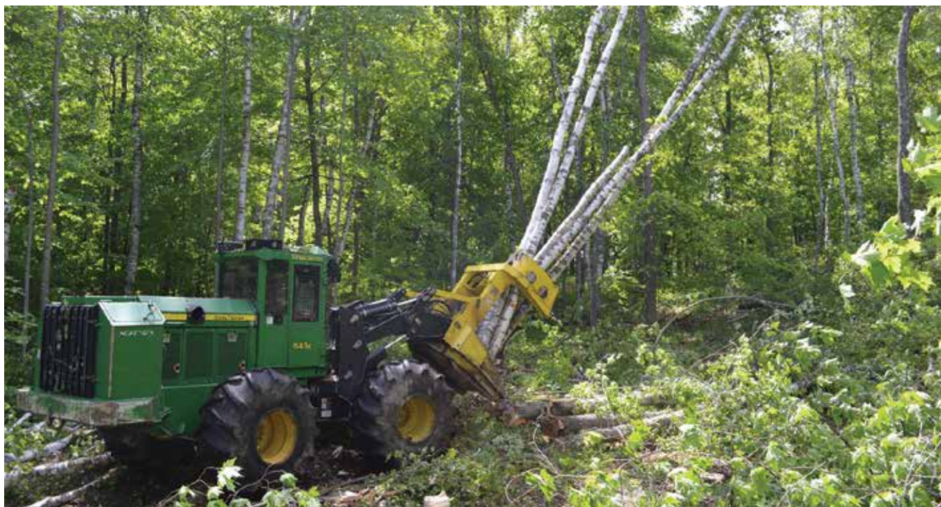
Steve Loch runs Dukek's John Deere 643K feller buncher. Dukek also has a Timberpro 725 buncher that typically operates on hilly or softer ground.
