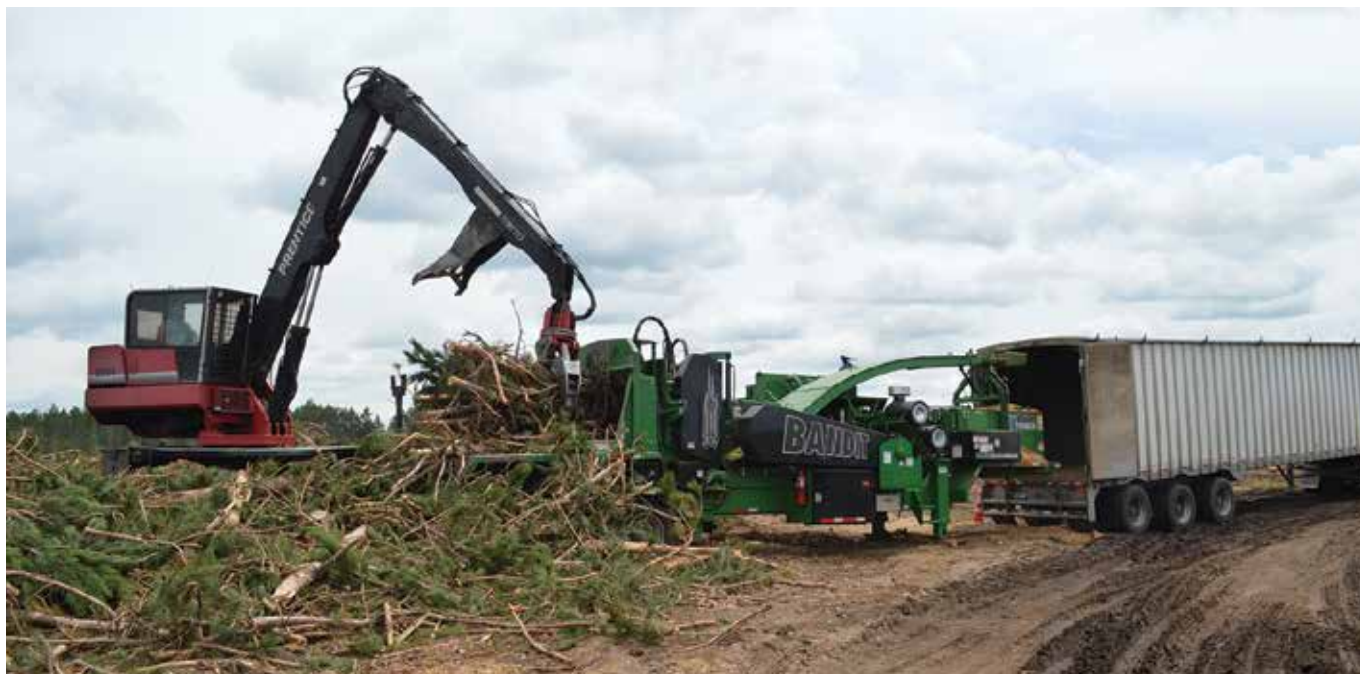
Mike Geller, chipping crew foreman, in another Prentice 384 loader—this one without a slasher—feeds Dukek's Bandit 3090 chipper at the Ainsworth red pine harvest.
