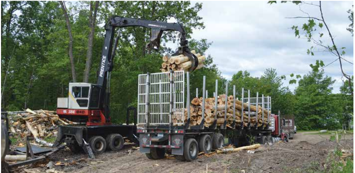
Dean Cluff loads a waiting truck with aspen with a Prentice Loader. Dukek Logging utilizes three Prentice 384s, two of which are equipped with slashers. Cluff also serves as Dukek's conventional crew foreman.
