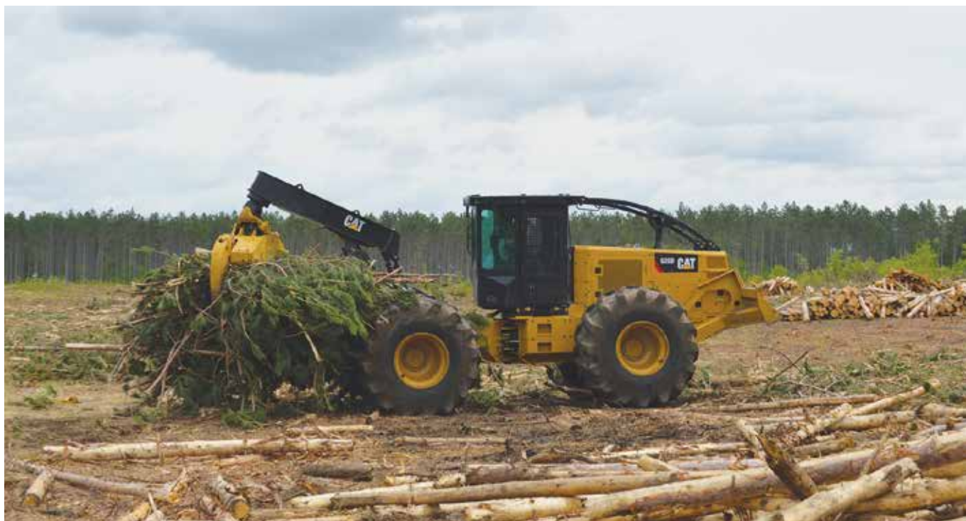
Doug Jacobs carries tops and limbs with a Cat 525 to Dukek's chipper at the red pine harvest at Ainsworth, Bemidji.
