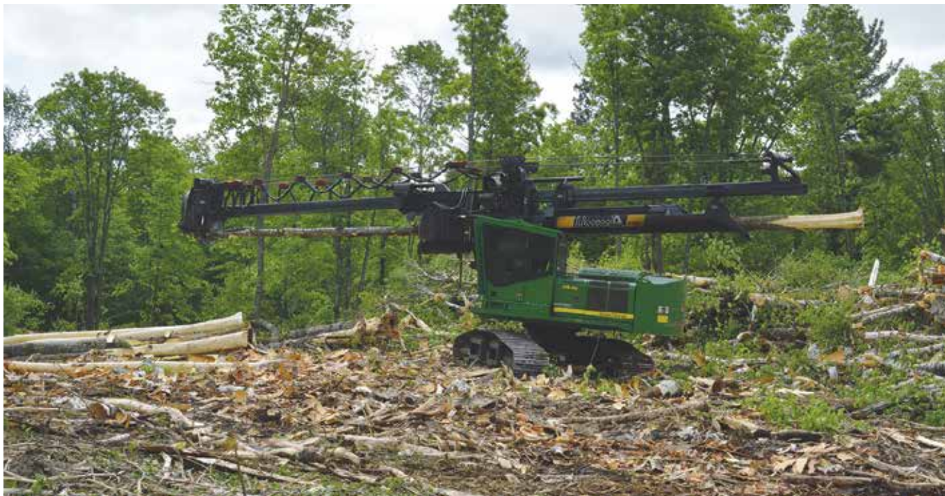
Jack Martine operates a John Deere 2154D stroke delimber with a 2100C Lim-mit at Dukek Logging's hardwood site near Longville.
