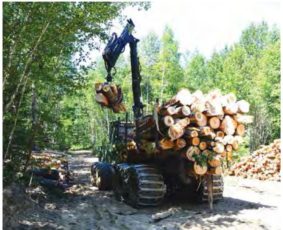
Scheff logging also operates three cut-to-length logging crews. Here, after aspen is harvested with a cut-to-length processor, a John Deere 1270D forwarder is used to pile the wood on the landing.
