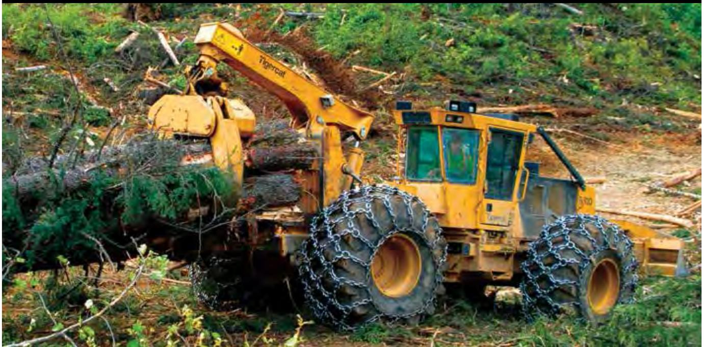
With Turnaround, the operator can comfortably drive the skidder blade-forward or grapple-forward while controlling all machine functions. In addition, the full infinite range of travel speeds and full maximum tractive effort are available in either direction at any engine speed, including low idle. No other skidder has these performance capabilities.
