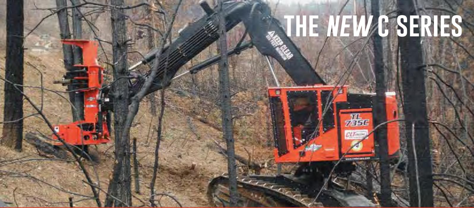
**THE NEW C SERIES FEATURES:** Hydrostatic swing, improved cab with taller windows, new style joystick pods, improved serviceability
