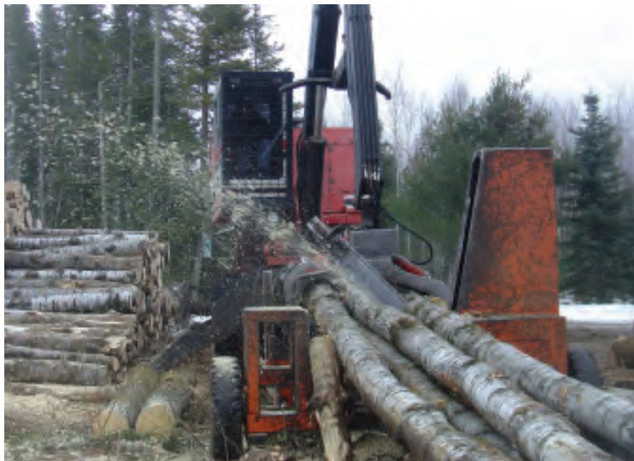
Ron Krueth operates the Prentice loader-slasher. To produce the 11-footers needed for the Helblad mill, the Krueths use a slasher with a bar saw. They also have a slasher with a more common 72-inch Serco saw on a Lemco XL280 loader when higher production is needed.
