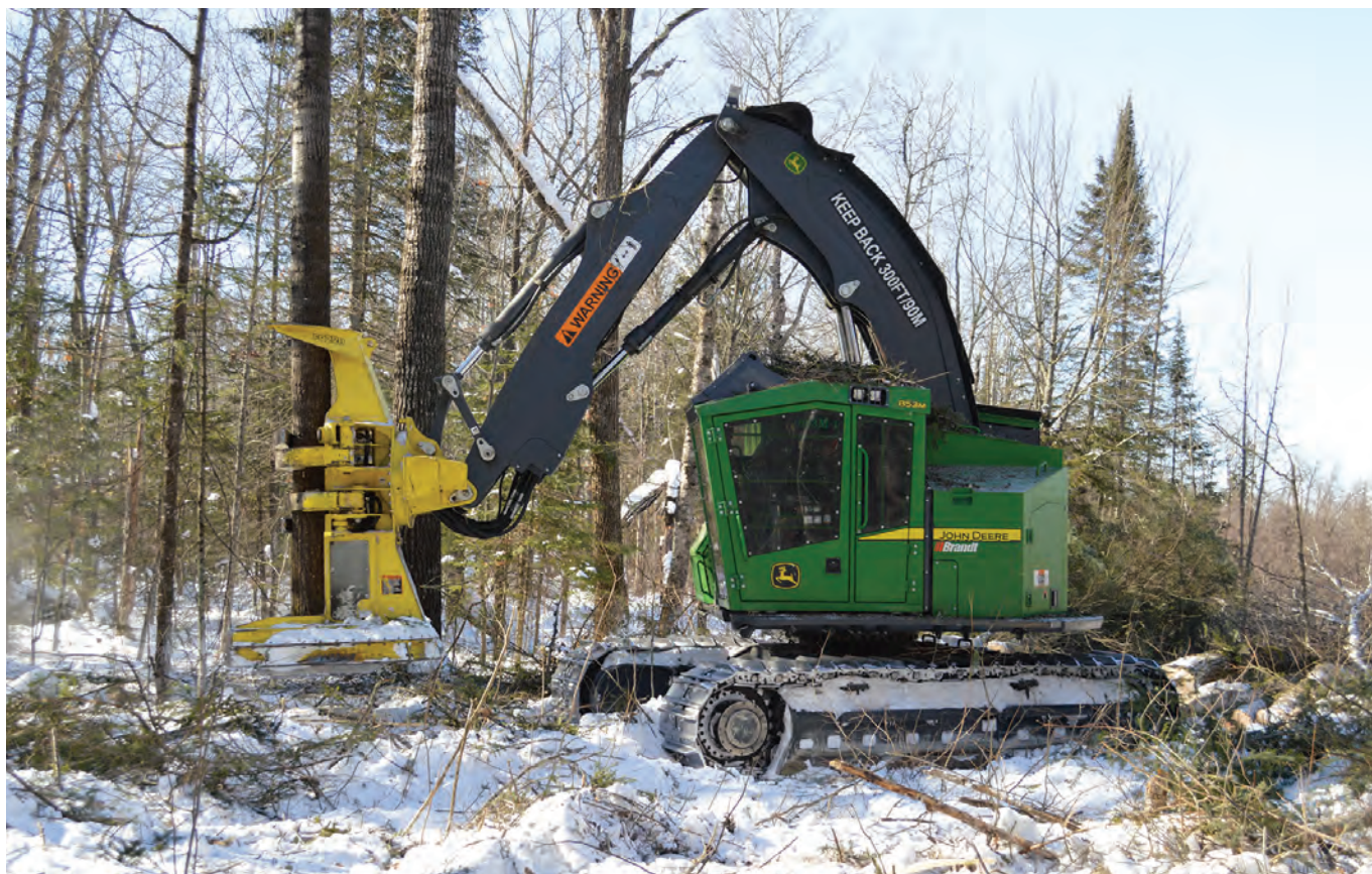
Eric Nistler harvests aspen with a John Deere 853M feller buncher at a harvest site north of Palisade.
