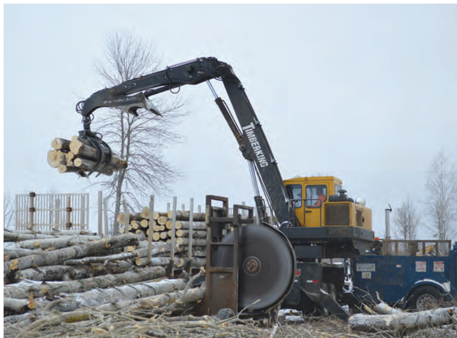
Tony Kowitz loads a crib trailer with 100-inch sticks of aspen. What isn't chipped, is either slashed into 100-inch lengths, or stockpiled tree-length.
