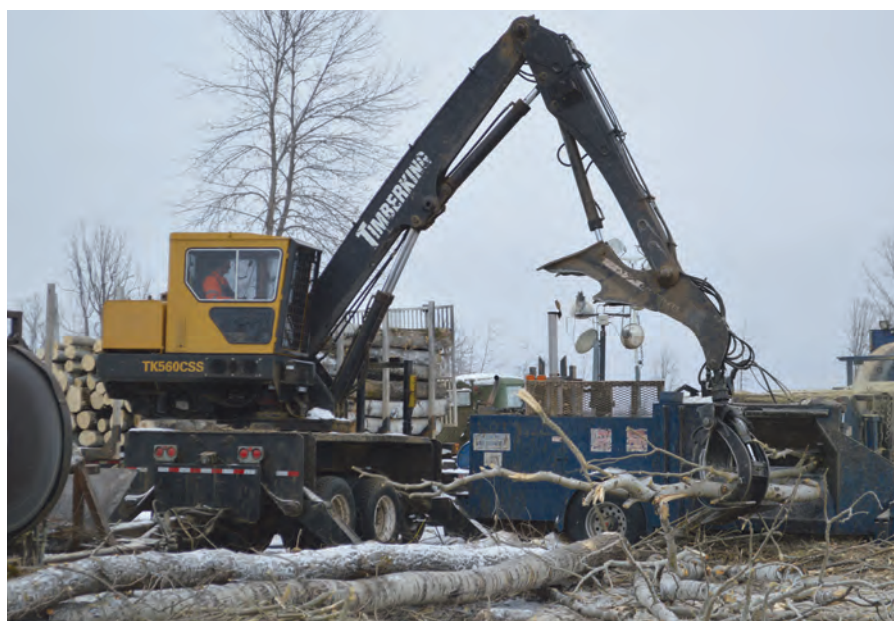
Tony Kowitz inserts harvested timber into the flail of a Peterson 5900 chipper. The flail removes barks and limbs, allowing for the production of clean chips.
