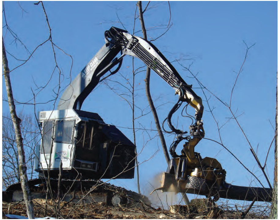
Tyler Hodgden harvests aspen in a Timbco 415D processor with a Fabtek FT 240 dangle head.
