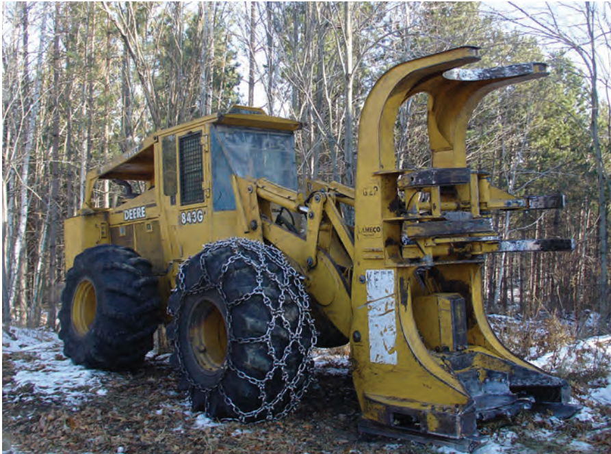
With harvesting operations on this sale nearly complete, the Hodgden John Deere 843G Feller Buncher waits to be moved to the next job.
