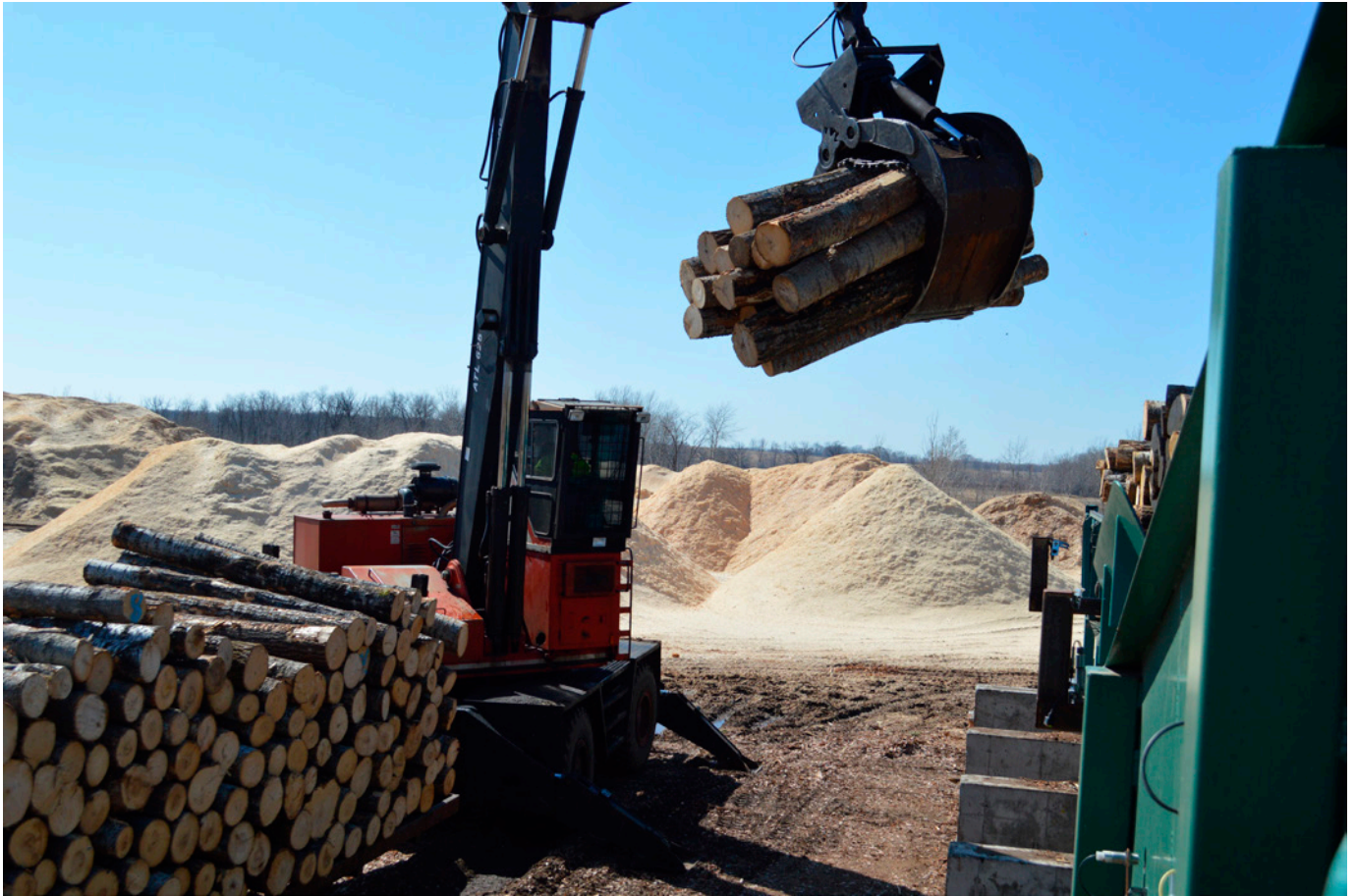
Harvested aspen is loaded onto the feed deck of the ring debarker.
